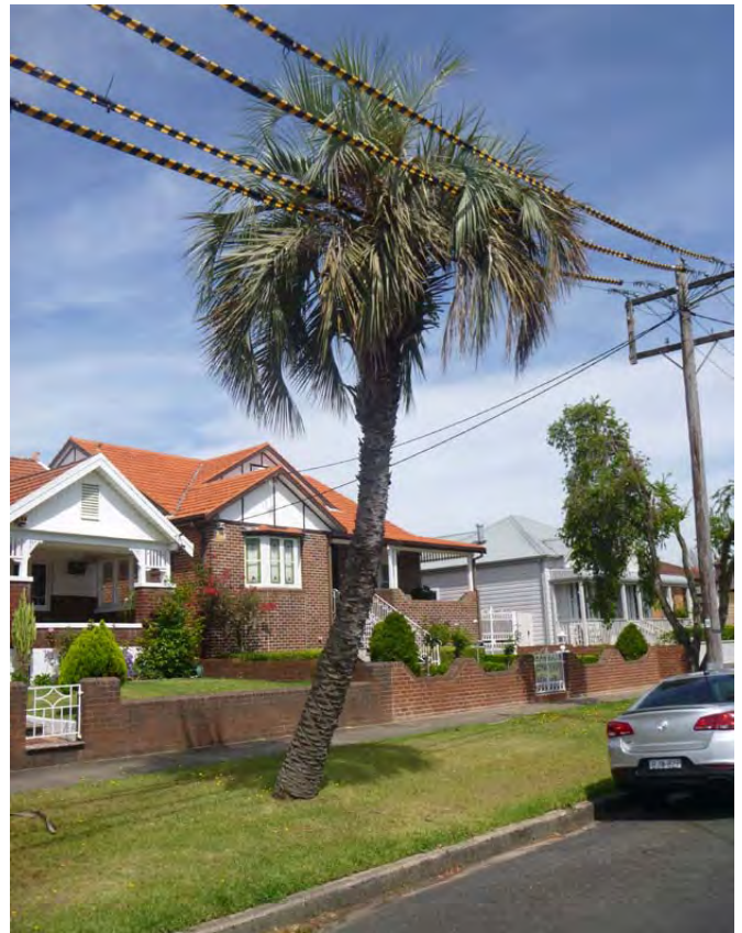
Figure 2.31- Martin Street, Dobroyd Point- it has taken almost 100 years but now even the slow growing Jelly Palms are causing an issue. A good approach is to transplant these to other areas or undertake ABC. (Photo-Arterra)
